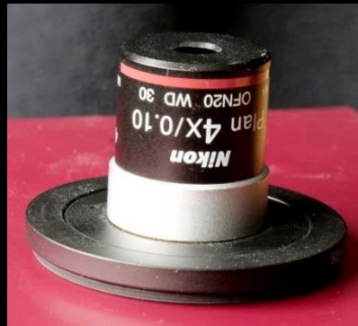
1x, 4x microscopic lenses \infty -corrected, Adapter: RMS \rightarrow 52mm
